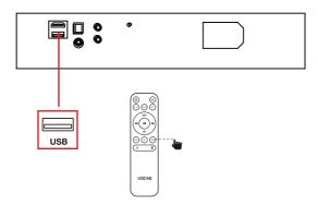
**Note**: USB interface: Supports USB1.1(FS). Support disk format: FAT32. Capacity: ≤ 64G (larger storage will affect loading time).In the future, upgrades can be made through the USB port.
